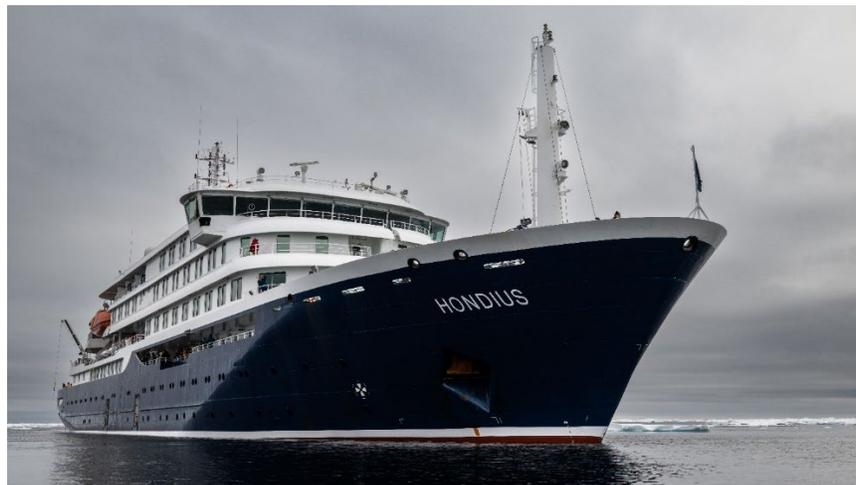
Hondius was built in 2019 in Split, Croatia. She is 107.6m long, 17.6m wide, and has a maximum draught of 5.3m. With an ice class of PC6, a top speed 15 knots, and three diesel generators, she sails on low sulfur marine gas oil and has a capacity of 176 passengers in 83 cabins. This beautiful mid-century modern vessel is designed from the ground up for polar adventure.
