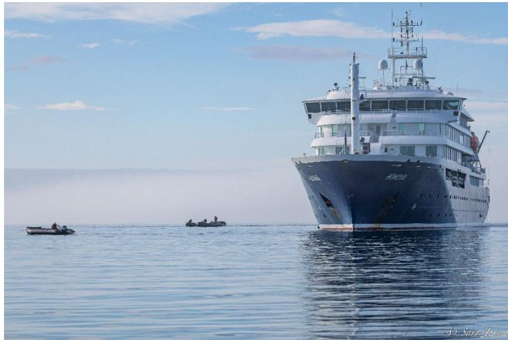
Hondius was built in 2019 in Split, Croatia. She is 107.6m long, 17.6m wide, and has a maximum draught of 5.3m. With an ice class of PC6, a top speed 15 knots, and three diesel generators, she sails on low sulfur marine gas oil and has a capacity of 176 passengers in 83 cabins. This comfortable, structurally advanced vessel is built from the ground up for polar adventure.
